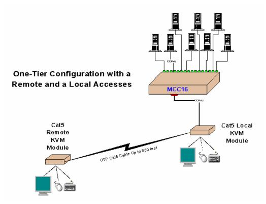
Figure 31 One-Tier with Remote Access Kit
